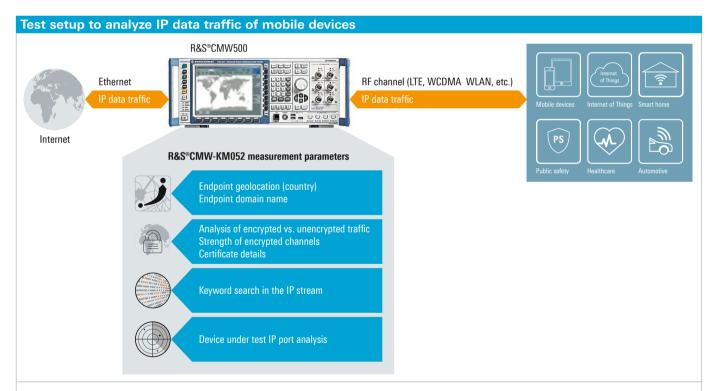
The R&S°CMW500 wideband mobile communication tester with the R&S°CMW-KM052 IP connection security analysis option enables users to identify vulnerabilities in an IoT device's IP connection security at an early stage of development.
