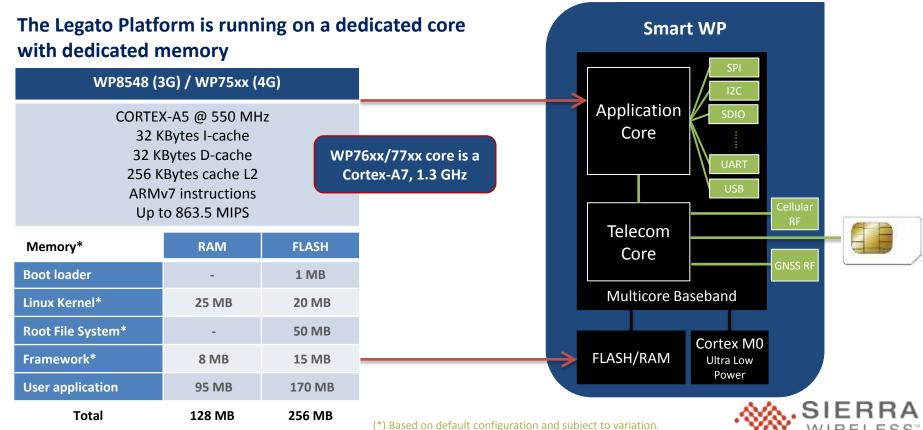
Code is executed in RAM. The telecom core uses a separate memory area.
